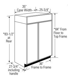
\* Shipping height. The refrigerator can be adjusted to fit into a cutout that is 83-1/2" min. to 84-1/2" max. height Note that the top case trim at the front is 1/2" higher and will overlap upper cabinetry or soffit. Use leveling legs and wheels for a maximum 1" height adjustment.
